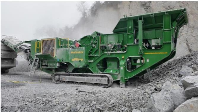
Efficiency is boosted with the new crusher design, particularly in the material flow path. Each sectional component is wider than the last to allow an unrestricted flow without funneling or narrowing, eliminating material bridging. The straight sided chutes manage the material as it passes through each section that is wider than the
